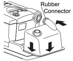
3. Connect the flexible tubing to the outlet port on the water chamber. If pressure tubing is used with your CPAP device, connect the pressure tubing to the pressure outlet on the front of the CPAP device.
