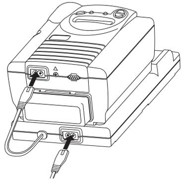
3. Place the CPAP device and humidifier platform on a firm, flat surface at a level lower than your sleeping position.
