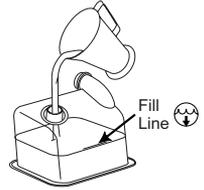
**CAUTION!** Do not allow the water chamber to sit for any length of time after it has been filled with water. Immediately install the chamber into the humidifier (step 2). Allowing water to sit in the chamber (when it is not connected to the humidifier) may cause the chamber to separate from the bottom plate and water leakage.
