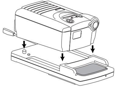
2. Connect the humidifier's power jumper cord to the AC inlet on the device. Plug the CPAP device's power cord into the AC connector on the humidifier. Plug the remaining end of the power cord into an AC outlet.
